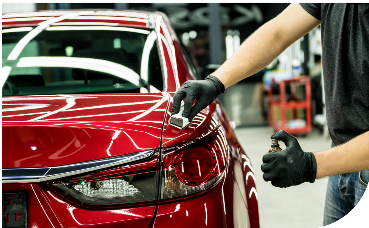
Fig. 3. One use of primary nanoplastics is in scratch resistant coatings. Source: Roman Zaiets, Shutterstock
